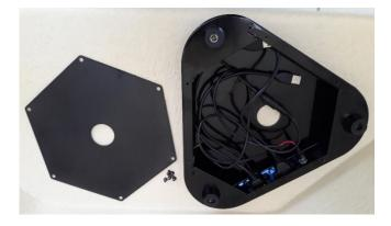
Unscrew and remove the cover from the bottom of the base.
