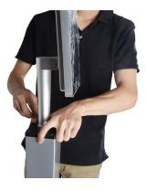
Seat the display unit head on top of the pole and tighten the 4 screws to secure the display unit to the pole.
