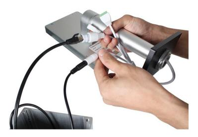
Connect the Ethernet and power ports from the display unit to the corresponding cables from the pole. Disregard the two cables with green ends, they are not needed immediately and are used only for Wiegand and Relay interfaces.
