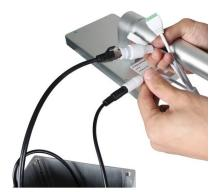
Connect the Ethernet and power ports from the display unit to the corresponding cables from the base unit. Disregard the two cables with green ends, they are not needed immediately and are used only for Wiegand and Relay interfaces.
