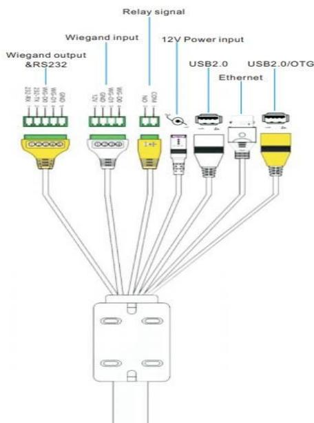
The Wiegand input and output interfaces can be used to control entry gates that use the popular Wiegand protocol. The Relay interface is used to control other devices based on the temperature monitoring results. Ethernet and USB ports can be used to connect the scanner device to other computing devices.
